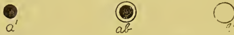
FIG. 24.—SHOWING THE APPEARANCE OF THE COMBINED STEREOSCOPIC IMAGE ab BETWEEN THE UNCOMBINED CROSSED NON-PLASTIC PICTURES a' AND b' PROJECTED FROM THE RIGHT AND LEFT EYES RESPECTIVELY.
